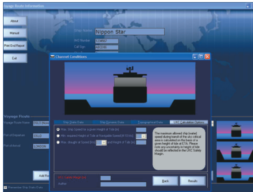
Screen shot from Nautical Technology Consultants new UKC Voyage Planner software. The program can help to prevent grounding in shallow waters.
